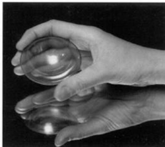
Fig 5 CVD diamond hemispherical dome, 75mm diameter and 2 mm thick
